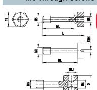
Titanium and Stainless steel screws create more options for mounting and adding additional styli. Check Lengths to match with cube size.
